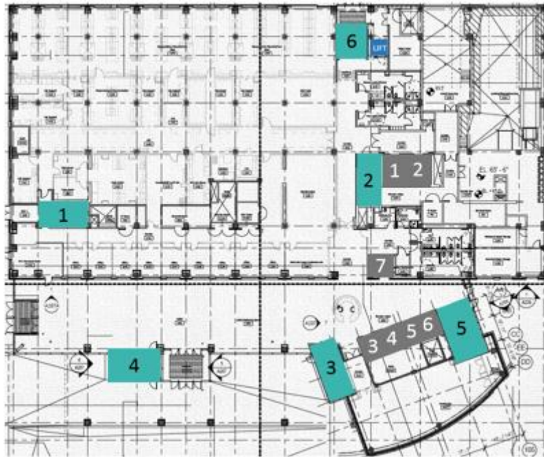
Figure 7: Layout of Stairs and Elevators
